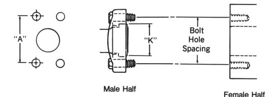
\*ISO/DIS 6162, DIN 20066, JIS B 8363, JIS B 8363 Komatsu Flange, and SAE J518 are interchangeable, except for bolt sizes.
